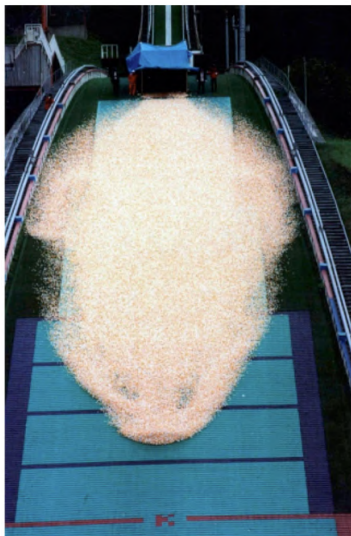
Figure 18 – Outdoor experiment of granular flow utilizing 300000 ping-pong balls at the Miyanomori ski jump hill in Hokkaido, Japan.
